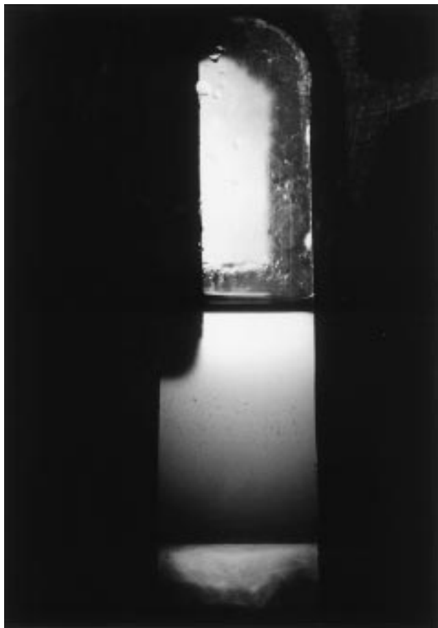
Fig. 11. SLV equilibrium in the \text{NH}_3\text{-H}_2\text{O-NaOH} system at 303 K and 0.7 MPa; initial concentration of NaOH, w_{0,\text{NaOH}} = 20 mass %.
